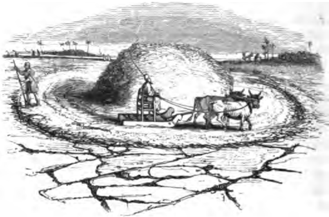
VIQUETTE F.—The Nôreg, a machine used by the modern Egyptians for threshing corn.
